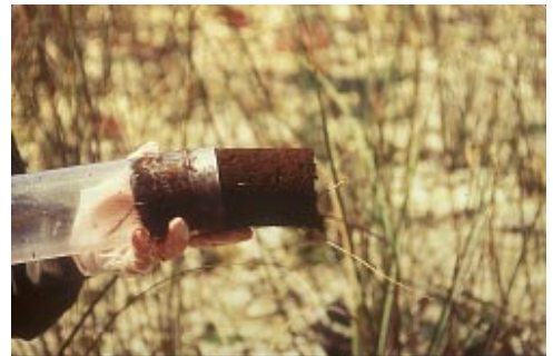
Figure 12. Soil cores were collected at each of the marsh sites and analyzed for mercury, nutrients, and other constituents.
