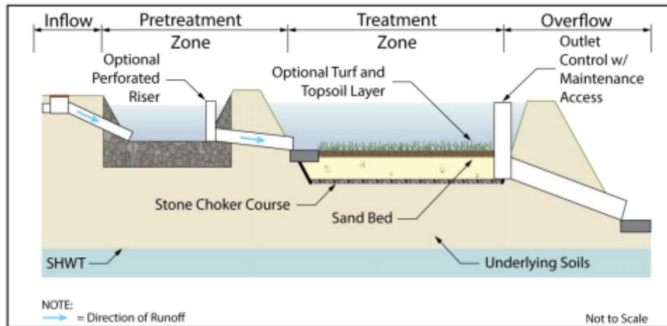
Figure 16. Sand Filter schematic. (Source: NJDEP 2021)
