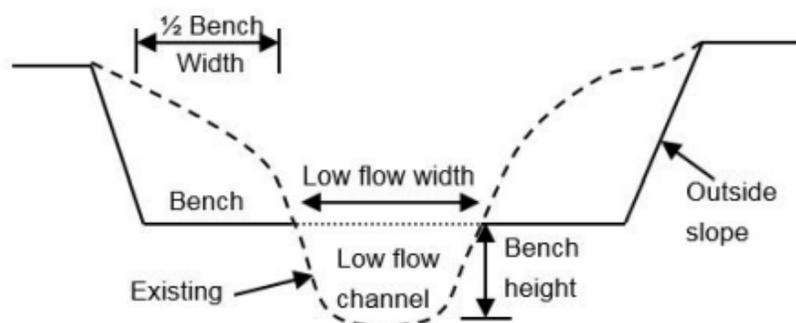
**Figure 9. Illustration comparing a conventional ditch (*dotted line*) and a two-stage ditch (*solid line*). (Source: NRCS, Indiana 2018)**
