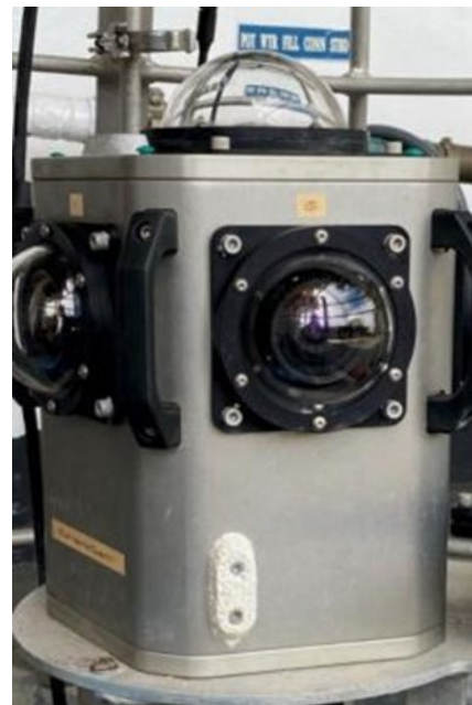
Close up view of the camera system with multiple fisheye lenses. (Photo courtesy of NOAA Fisheries).
