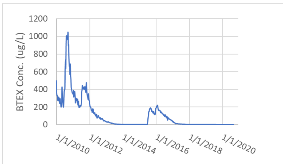
Figure 3. Influent BTEX Concentrations Over Time
