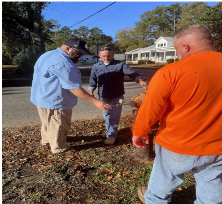
Chad Byars and Phil Franklin of SCWRA and Mayor Garner, Town of McColl, flow-testing hydrants.
