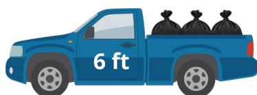
$$\begin{array}{l} 6 \text{ ft} \times 5 \text{ ft} \times 1.5 \text{ ft} = \\ 45 \times 10 \text{ loads}/27 = \\ \hline 17 \text{ CY} \end{array}$$
