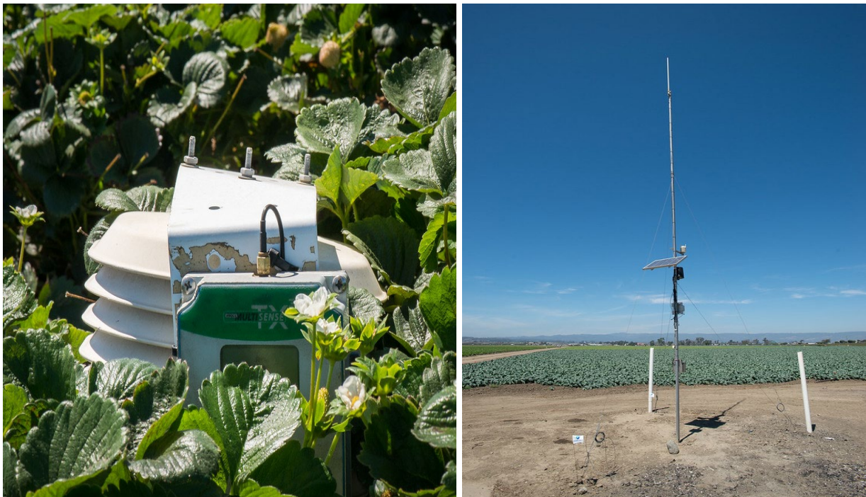
Figure 12. Wireless soil tensiometers in the field along with a solar-powered weather station monitor field conditions for an irrigation water management system in California. Photos by U.S. Department of Agriculture.
