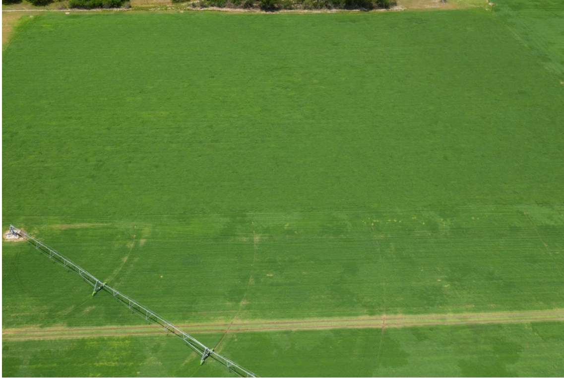
Figure 15. Subsurface drip irrigation (top half of picture above) and center pivot irrigation (bottom half of picture above) systems with runoff controls irrigate hayfields in Texas. Photo by U.S. Department of Agriculture.
