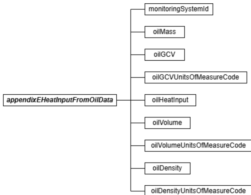
Figure 33: appendixEHeatInputFromOilData JSON Elements
