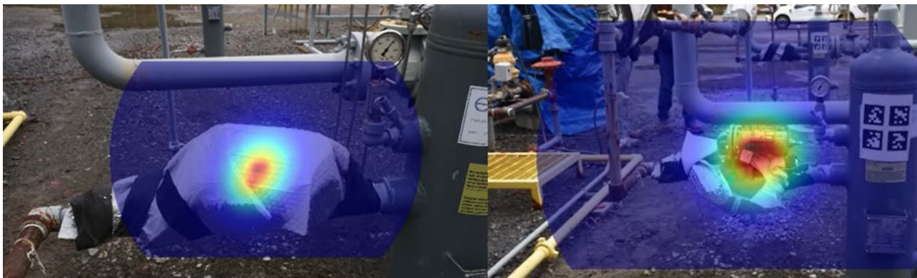
Figure 2. Examples of emission detection from a regulator under bubble wrap. On the left, methane emission visualization shows emission coming from under bubble wrap. On the right, a Digital Emission Tag for the regulator is created once the bubble wrap is removed. Removing bubble wrap is required to localize the emission to the specific component under the wrap.
