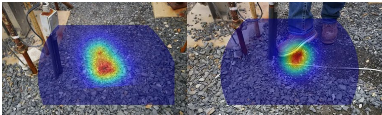
Figure 3. Example of emission detection from a buried tubing connector. On the left, methane emission visualization shows methane emission coming from the ground. On the right, a Digital Emission Tag for a connector on buried tubing is created once the gravel is removed.
